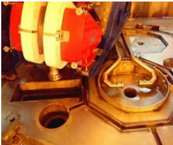
Fig. 18. View of the bending part of the transportation channel that is ready for the NGT installation (turned at 45°)
