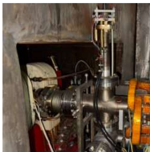
Fig. 5. Connection unit of the horizontal and bending part of the accelerator vacuum system
