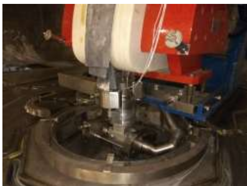
Fig. 7. Connection unit of the bending part and NGT vacuum chamber
