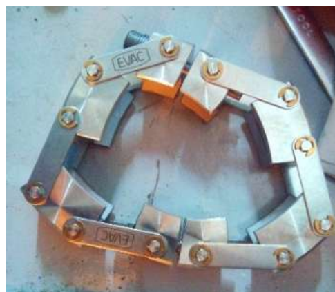
Fig. 6. Fast released vacuum clamp to connect horizontal and bending part of the accelerator transportation channel vacuum system
