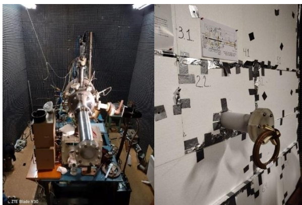
Fig. 1. General view of the DAEA DIN-2K with no interference-absorbing screen (photo on the left) and with a screen
