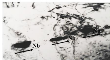
Fig. 5. Intermittent distribution of niobium layers in cast metal (electron microscopy)
