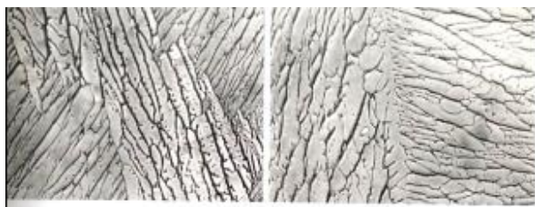
Fig. 3. Microstructure of Zr1Nb alloy ingots after electron beam remelting, x500
