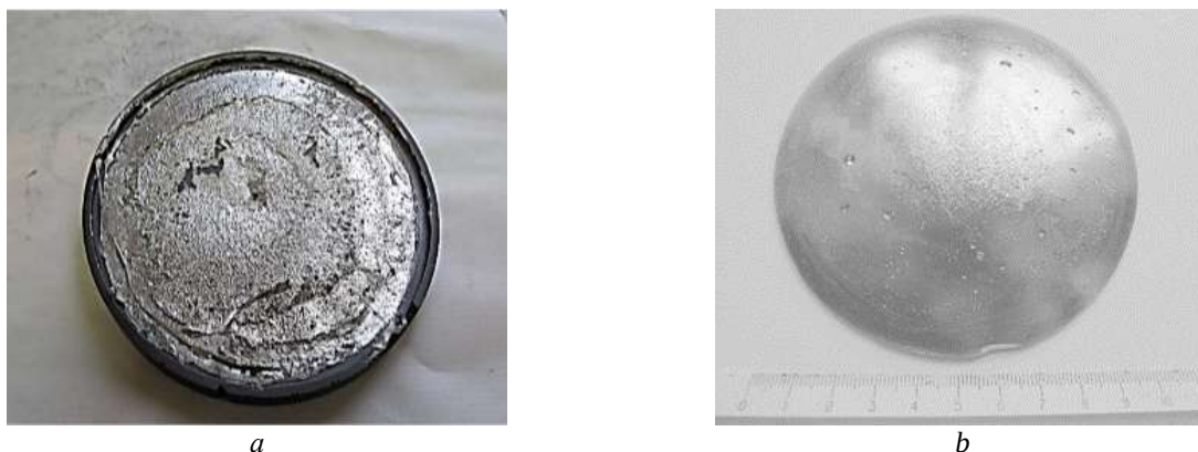
Fig. 4. Collected oxide contaminants after filtration of the initial zinc (a) and filtered zinc (b)
